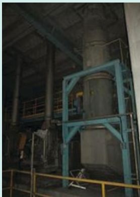
All chopped glass fiber products are dried using only waste heat
