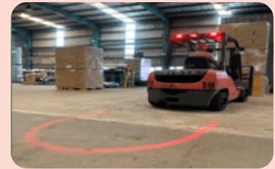
Forklifts are equipped with arced LED lights
